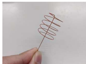
NiTi wire with shape memory treatment (with PTFE coating)
