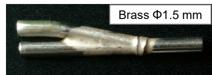
Brazing (Another pipe is brazed to the top of the main pipe)
