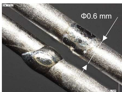
Soldering (joining NiTi pipes)
