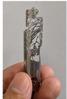
Processed sample cut into Maiko's shape (14 mm OD × 13 mm ID)
