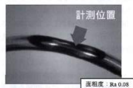
Fig. 7 Inner surface of elbow part after slurry flow polishing.
